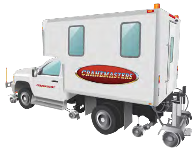
The Cranemasters Puckett TLV Truck (Track Loading Vehicle) inspects both static gauge and loaded gauge in one pass. Learn More >
