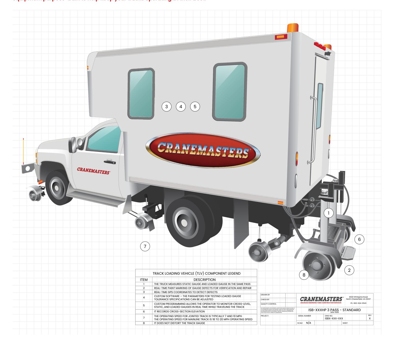
The TLV has been inspecting railroad tracks for over twenty years. You may know it as the 'Puckett Truck.' Its custom programming can monitor cross-level, static, and loaded gauges in real time as it travels your track.
