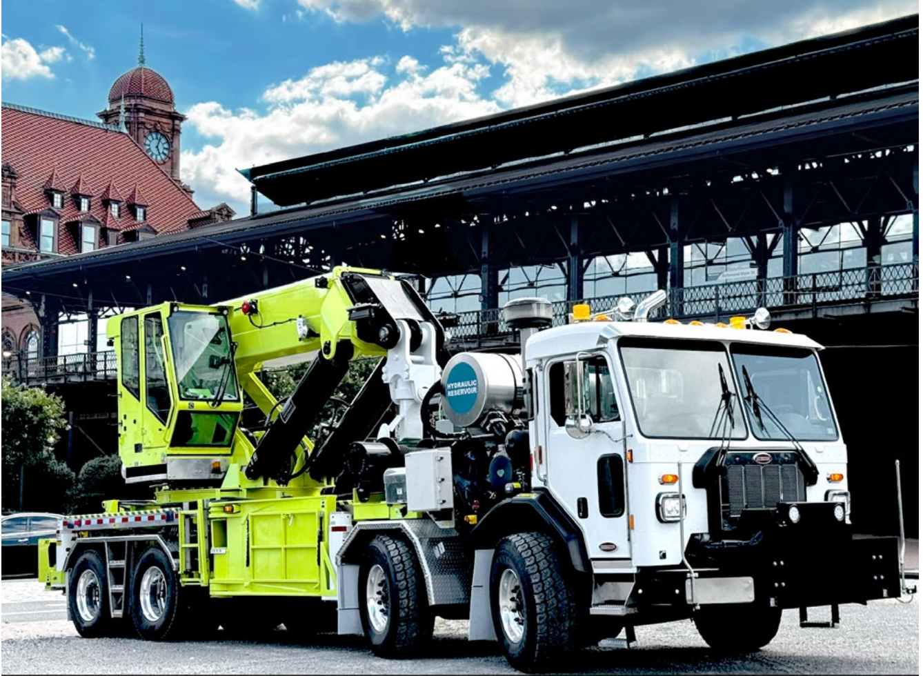
The Cranemasters CMD130R with a short, telescoping boom and a fixed hook
